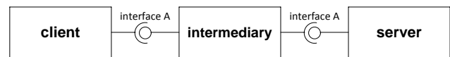
Figure 4: An instrumented connector has an intermediary component in the connection between client and server.
